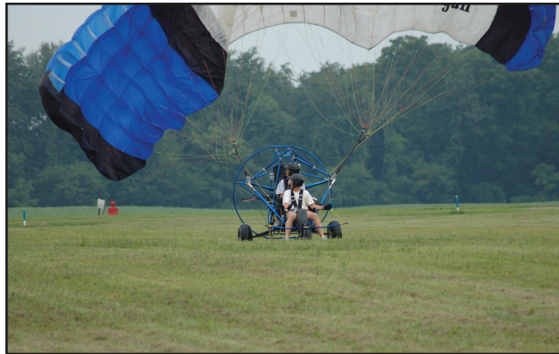
Figure 11-7. Collapsing the parachute.
