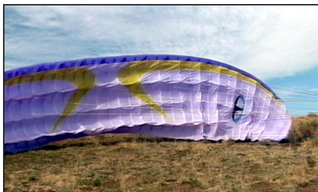
Figure 12-3. A wing wall.
