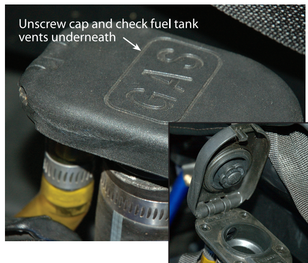
Figure 5-9. Inspect that the fuel tank vents are free of dirt and debris to prevent fuel starvation during flight.
