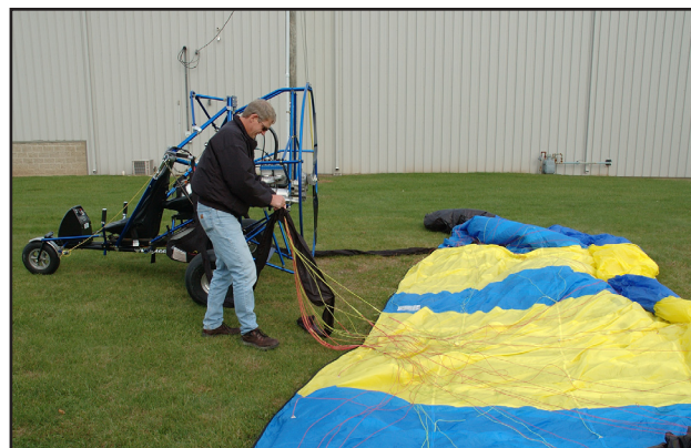
Figure 5-15. Removal of the line sleeve is an important step in the wing layout and inspection.
