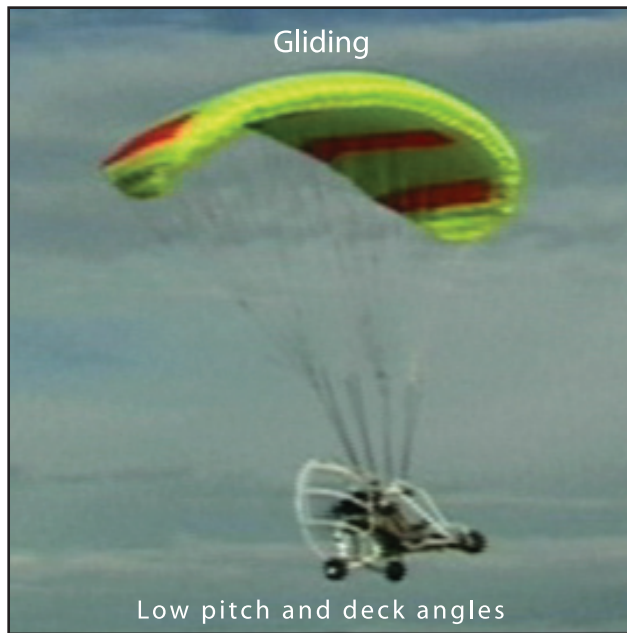
Figure 2-4. Gliding and climbing pitch angles.
