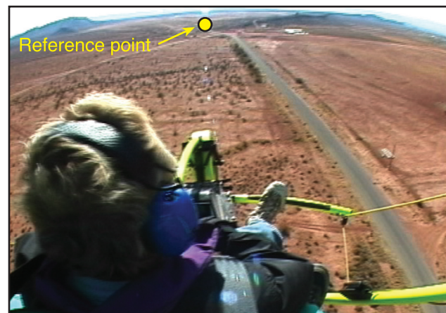
Figure 6-4. Nose reference for straight-and-level flight.
