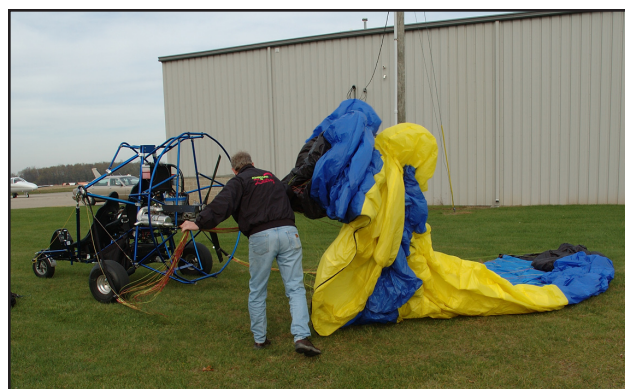
Figure 5-19. Undoing a line twist—beginning of the process.
