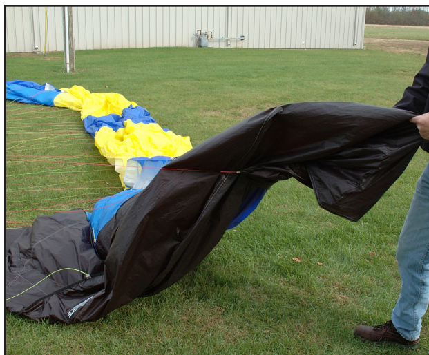
Figure 5-21. A simulated line-over.
