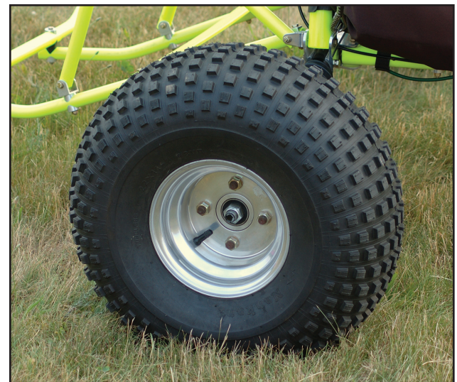
Figure 3-19. Some powered parachute tires are heavily treaded while others are smooth.
