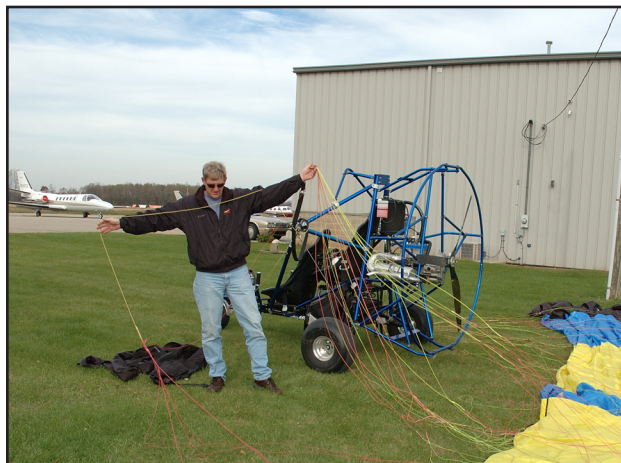
Figure 5-16. The pilot will physically pull the steering lines out and away from the bundle of suspension lines to ensure they are tangle free.
