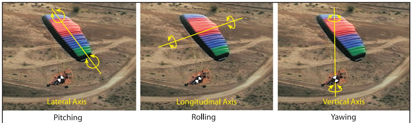
Figure 2-18. PPC axes of rotation.
